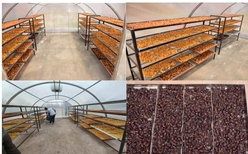
Fig. 4. Date palm drying in a large-size tunnel-type PV/thermal hybrid solar dryer
