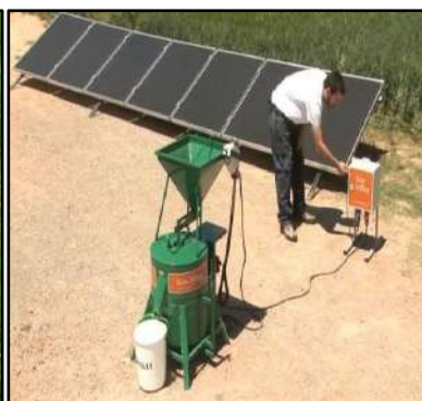
Solar powered mill
