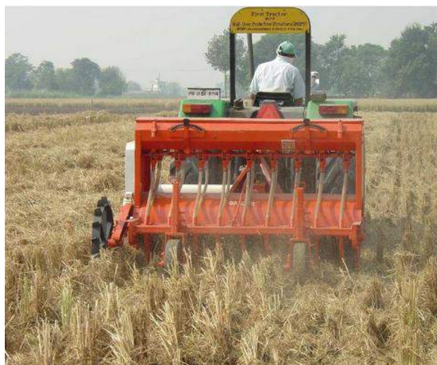
Figure 1. Sowing wheat into rice residues with happy seed drill (Source: Sidhu et al. , 2015)
