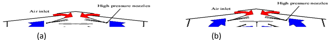
Schematic view of the prepared system (a) Forced ventilation and (b) Natural ventilation
