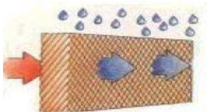
Cooling livestock buildings by Pad and Fan Evaporative Cooling System (Pad Cooling)
