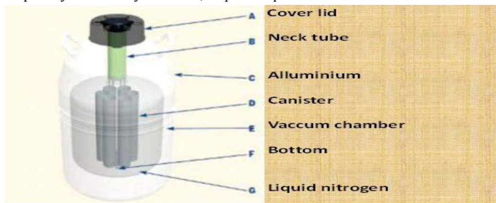
Figure-2. Internal structure of Liquid nitrogen container. *Photo source: Internet
