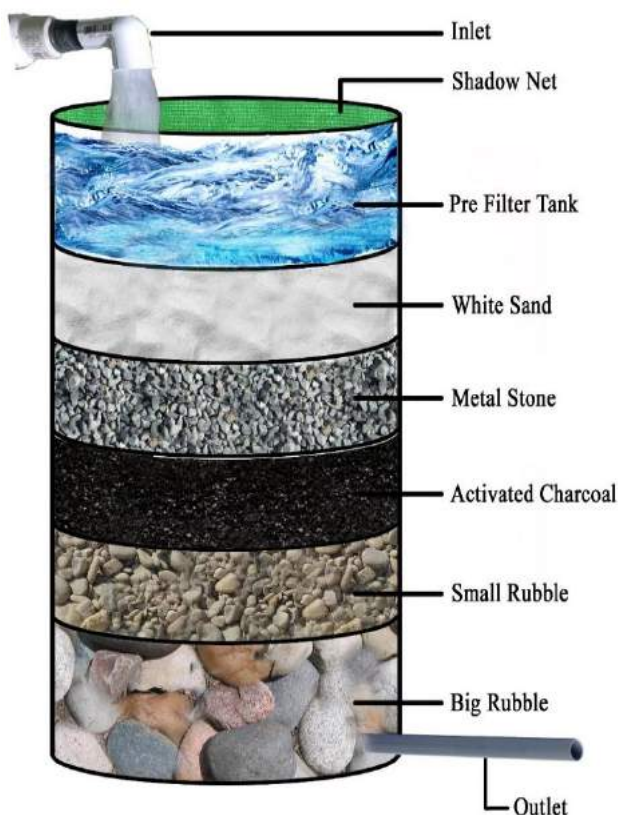
Fig. 1 A cross-sectional diagram of a sand filter
